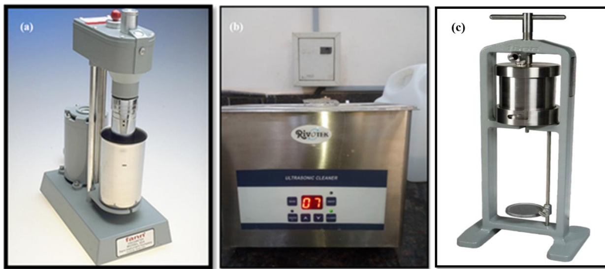
Figure 5.1 (a) Fann VG meter, (b) sonicator shows two step method for nanofluid preparation and (c) API filter press.
